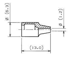
Figure 10 #3-4 Hood (for Ø0.9 mm buffered fiber)
