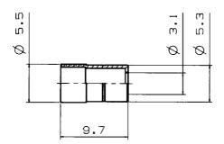
Figure 5 #2-1 Crimping ring ( for ø3.0 mm cord )
