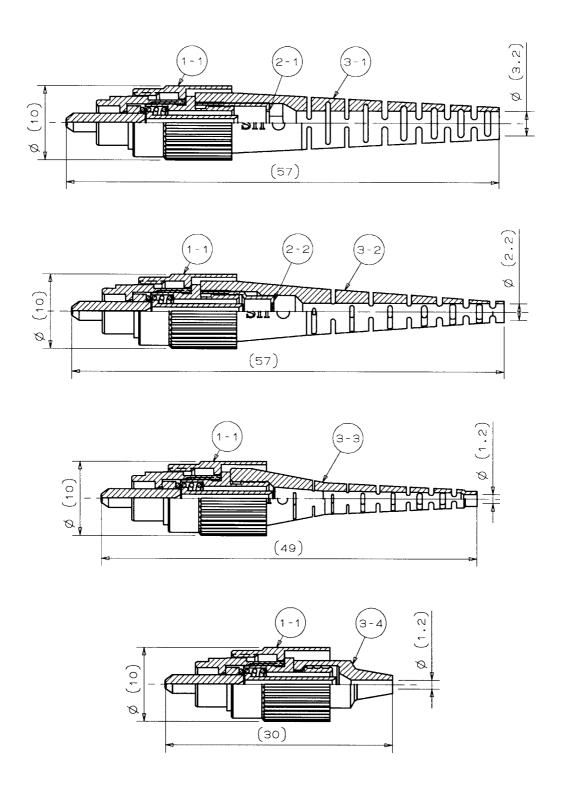
note 1: This drawing shows the tentatively assembled condition. In practice, the connector plug is not assembled like this. note 2: This drawing does not include the caps.
