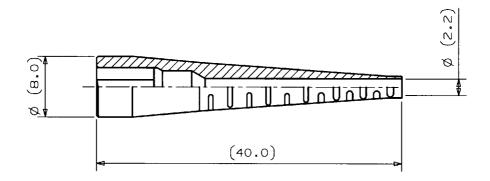
Figure 8  $\#3-2 \text{ Hood ( for } \emptyset 2.0 \text{ mm cord )}$
