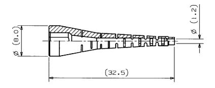
Figure 9 #3-3 Hood ( for Ø0.9 mm buffered fiber )
